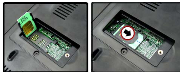
Figure 13 - Insert the USIM Card & Lock the SIM-LOCK
